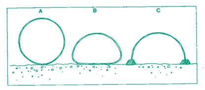
Three common types of stream crossing culverts are used in forestland road construction: A) round culvert; B) pipe arch culvert; and C) plate arch "culvert." For stream crossings where fish passage must be accommodated and a bridge cannot be installed, plate arch culverts are preferred. Round culverts are the least preferred culverting method where fish passage is important (from Handbook for Forest and Ranch Roads).
