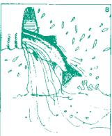
Incorrect culvert installation can impede or prevent fish passage through a streamcrossing. Culvert conditions that block fish passage include: A) water velocities too great; B) water depths too shallow; C) insufficient resting area or jumping pool depth at culvert outlet; and D) culvert outlets that are too high above the streambed (Furniss, et al. in Handbook for Forest and Ranch Roads).
