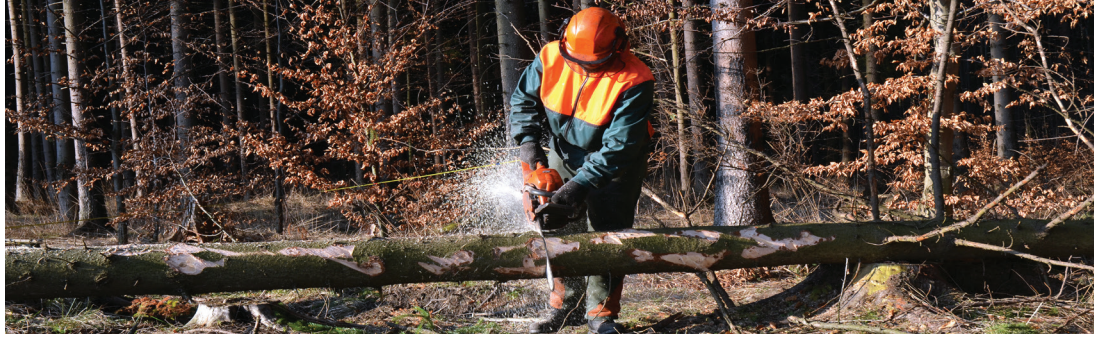
Protective clothing—chaps, pants, jackets, gloves, hardhats or helmets, face guards, hearing protectors and steel-toe boots—increase personal safety when operating power tools. Source: Adobe Stock
