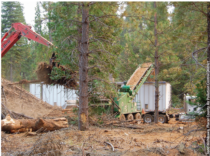
At Blodgett Forest Research Station near Georgetown, an excavator (left) loads forest slash into a horizontal grinder. Wood chips from the grinder go into trucks for transport to Buena Vista Biomass Power Plant near Lone (right). Source: CalAg
