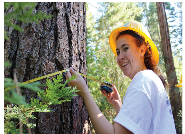
Alexis Flint, Golden Sierra High School team member, uses a D-Tape to measure the diameter of a tree
