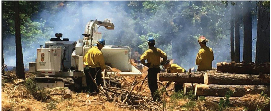
A crew chips slash during removal of dead trees in Sierra National Forest. Source: USFS
