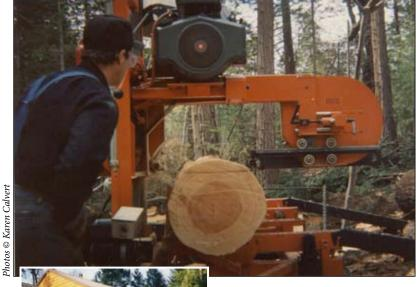
selected a bandsaw because of the type of material I wanted to produce, portability (only weighs 1800#), and cost. It was so easy to operate even a forester could do it! We have used it to build three homes, some garages,
