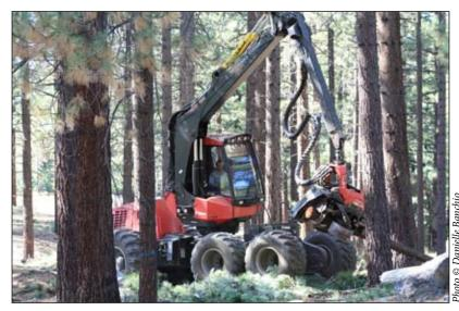
The harvester is a highly maneuverable, low ground pressure machine with a boom and head that grabs the tree, cuts it at the base, limbs it, and cuts it into the desired length. These machines are generally limited to 40-50% slopes.
